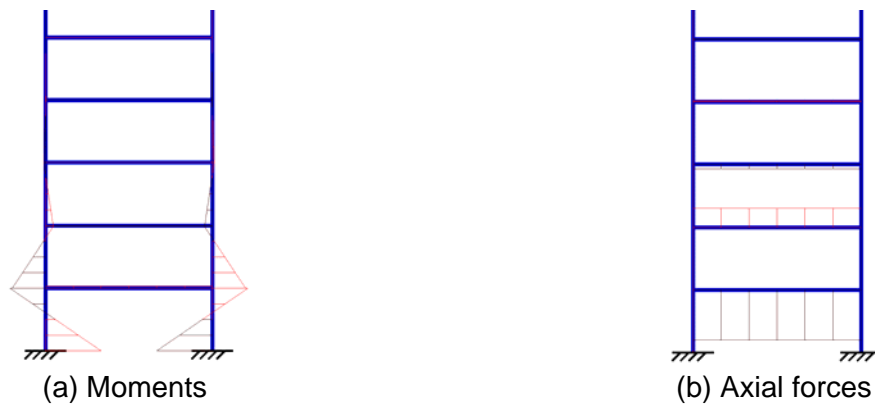
FIGURE 5 ACTIONS IN LOWER LEVELS OF A MULTI-STORY FRAME UNDER UNIFORM CHANGE IN TEMPEARTRE
